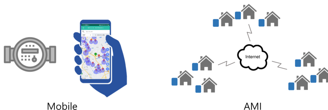
Figure 16. Water Meter Reading Method
